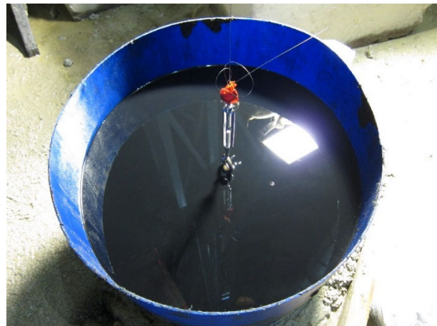
A heavy plumb bob with fins (left) and submerged in a container of oil during the observation (right).
