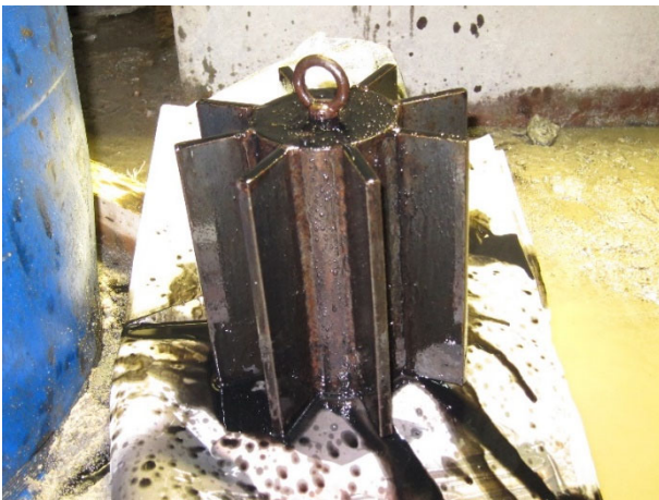
A heavy plumb bob with fins (left) and submerged in a container of oil during the observation (right).
