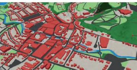
▲ Figure 2: Part of the 3D city model of Valkenburg, the Netherlands. Elements that can be represented in a 3D city model include: buildings, vegetation, water bodies, built-up areas, green areas, roads, etc. (Courtesy: Dutch Kadaster)
