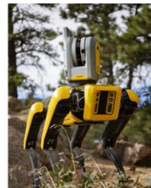
Boston Dynamics "Spot" platform with a Trimble X7 Scanner
